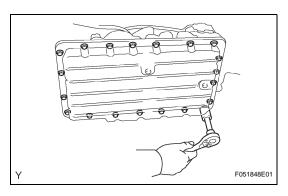
4. INSTALL AUTOMATIC TRANSMISSION OIL PAN SUB-ASSEMBLY
